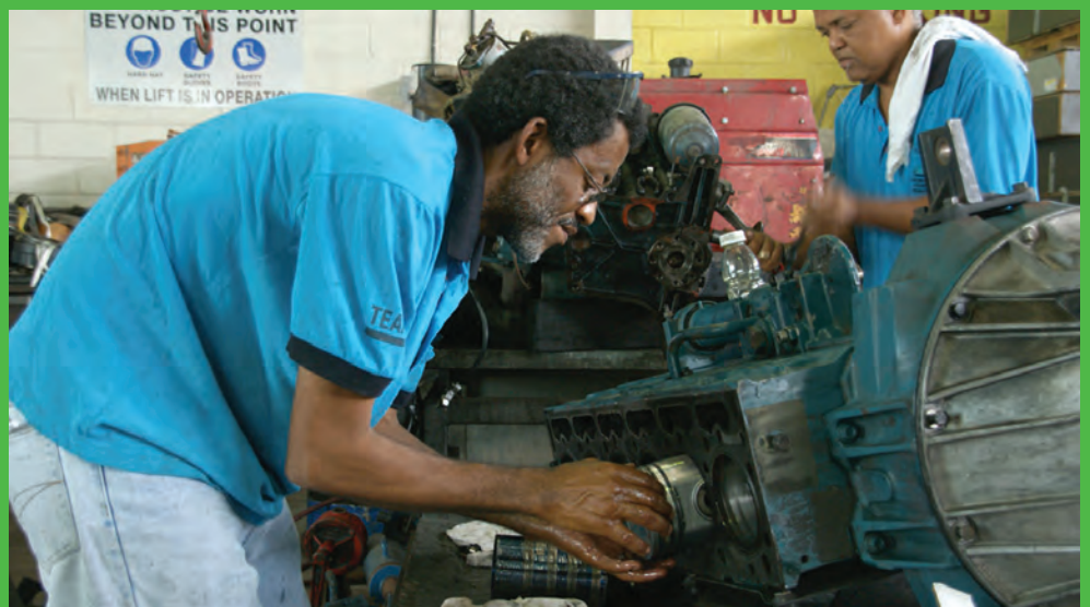
Stephen Brizan of the Transport Department fitting the engine to the newly converted CNG dump truck
