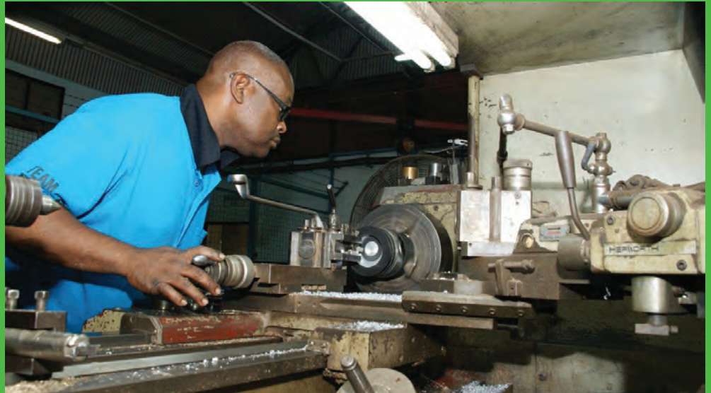
Kenny Brooks of the Central Workshop Facility in action as he uses the lathe machine to modify pistons as part of the conversion process
